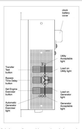
The digital controller provides sensing, timing, and control functions for the ATS. This micro-processor-based controller includes built-in control buttons and status lights for control of the ATS and the generator.
