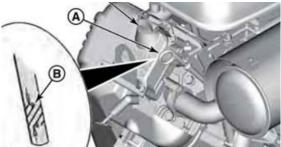
Oil is added to the engine by removing the oil cap and adding oil at this point. After filling the crankcase to the proper level, be sure you properly tighten the oil fill cap ('C').
